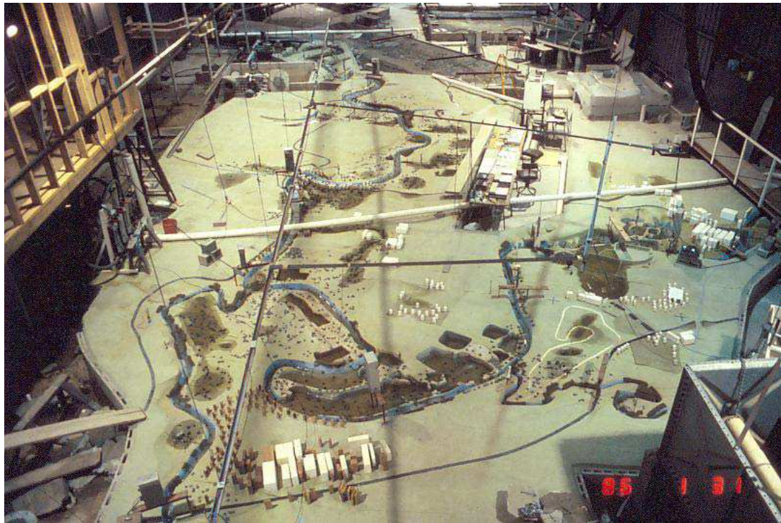
Figure 5.4 – Physical model of the upper reaches of the Georges River (WRL, 1991)
