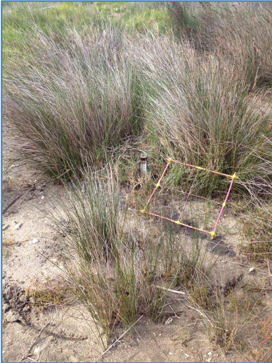
Figure 7 High reference category survey plot with 600 mm survey stake as centre point and 50 cm x 50 cm invertebrate survey quadrant.
