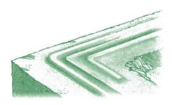
**Advantages.** There is a reduction in the amount of water that must be treated. The site is kept drier during wet periods.
