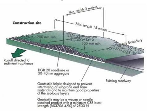
Where the entry/exit area slopes toward the road, a diversion hump should be installed across the stabilised area to direct stormwater run-off to the side where it can be filtered by a sediment fence.
